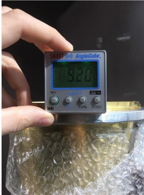
Move the level along the rim to find the point at which the angle is maximized. Compare this value to that read out in the angle tab. In any case click on the Show Data Manager icon, or press “D”.
